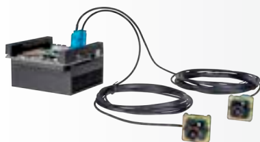
NVIDIA Jetson AGX Xavier shown with FPD-Link® III*
