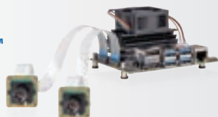
NVIDIA® Jetson Nano™ shown with MIPI® CSI-2*
