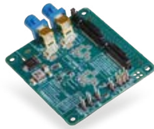
2-Channel FPD-Link III Deserializer for Development Kits With NVIDIA® Jetson Nano or NVIDIA Jetson Xavier™ NX (for Raspberry Pi)
